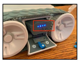
**Step 5**: Leave the battery charged until you see 4 blue dots NOT blinking. The four blue dots show that the battery is fully charged.
