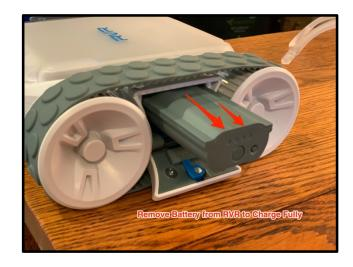
Step 4: The blue USB cord, included in your kit is used to charge the battery. It can be plugged into your laptop but can also be connected to an iPhone or iPad brick.
