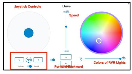
**Step 17:** This image shows the joystick controls. It also highlights other options that can be controlled using the Drive option.
