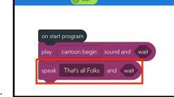
**Step 31:** The spoken text programming sound block speaks whatever you type into the block through the programming device.
